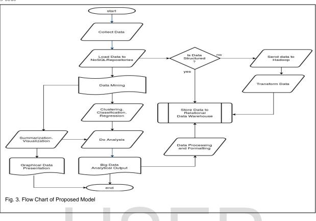
After processing data, processed data can be provide to data scientists or data researchers for analysis. Users can also receive processed data in graphical form. After analysis data, system provides big data analytical output. The output can be also stored in data warehouse by processing and formatting data. The flowchart is described as follows:
